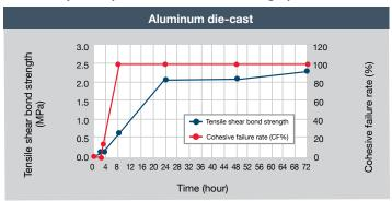
\* Bond line thickness: 1mm Cure condition: 1 week at 25°C
