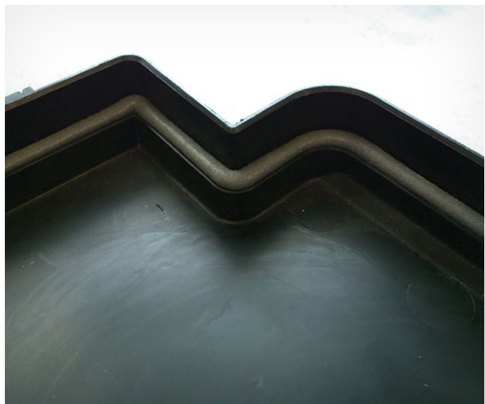
Figure 1. Robotic application of silicone foams speeds production and minimizes waste. These two-component silicone materials can be mixed either in static or dynamic mixers, though dynamic mixers are recommended to help ensure optimal density, cure and cell structure of the finished foam. Mixing produces a reaction that releases hydrogen gas as a foaming agent. The gasket expands in its liquid stage and cures to form a low-modulus, integrated compression seal. Seals are ready for handling as quickly as 10 minutes after application and can support full assembly within an hour at room temperature.
