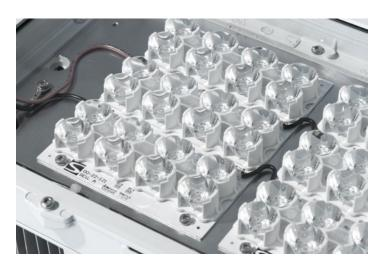
Using SILASTIC™ MS-1002 Moldable Silicone, the complex lens design, made of eight individual collimators attached together, was high precision injection molded, enabled by Gaggione. The silicone delivered outstanding mechanical, thermal and optical performances, and demolded easily.
