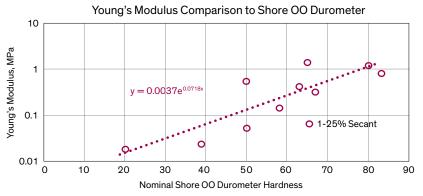
exponential curve fit also appears to fit very well to the data. Again, the DMA derived modulus is significantly higher than that from stress/strain curves (there was not enough RDA data available to plot).
