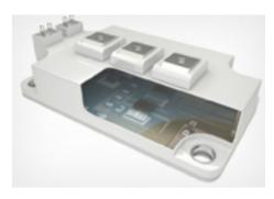
DOWSIL™ EG-3896 Dielectric Gel is a two-part, dielectric silicone that cures quickly with heat to form a tough encapsulant with excellent resistance to cracking and void formation. It offers strong self-priming adhesion to provide PCB system assembly modules with long-lasting protection against moisture, contamination and other environmental factors. The low modulus of this advanced
