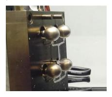
There are several different mandrels used for the interior of these globes; wall thickness varies from the neck to the tip. Much like metals can be made in wide flats for springs, or shaped as an I-beam for structural support, the variable cross section dramatically alters the feel of these globes.
