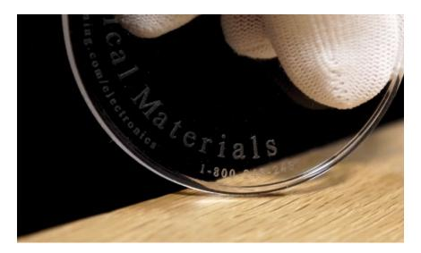
This shape was molded as a promotional item for customer visits. The disc is 68 mm (2.67 inches) in diameter and 3 mm (0.12 inches) thick in the center area. This mold is highly polished so it has a good optical surface and can be used for optical testing. The writing around the perimeter was etched
