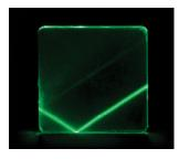
This shape was molded in response to requests for a larger and thicker plaque for optical testing. This mold is highly polished so it has a good optical surface; overall dimensions are approximately 50 mm x 50 mm x 4 mm (2 inches x 2 inches x 5/32 inches). The polished surfaces again work well to show internal reflection and can be used to show light extraction.
