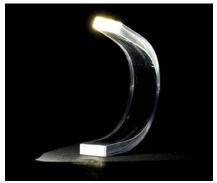
Finally, if a laser is placed at the end of the bar, and a light pipe cylinder is stood upright and pressed against it, light can be extracted along the cylinder. This light extraction is useful in some designs and can also be accomplished by roughening the portion of the mold where the light extraction is desired.
