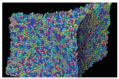
X-ray tomography of potting foam showing uniform cells
