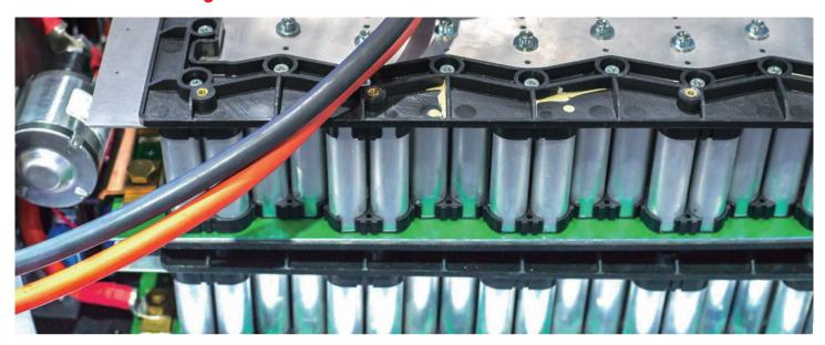
Reliability, ease of manufacture and good mechanical stability make cylindrical cell designs a popular option for hybrid/electric vehicle (H/EV) batteries. They typically burn less energy than pouch and prismatic designs, resulting in higher battery range, and can be very durable when utilized correctly. Of course, there's always room for improvement—and that's where we come in.
