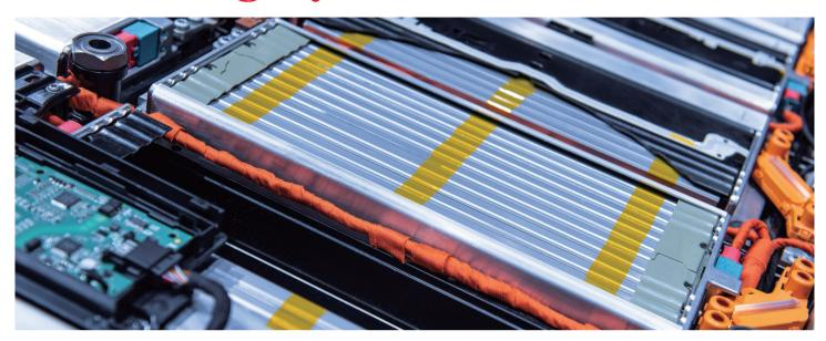
Virtually every hybrid/electric vehicle (H/EV) battery system uses some type of thermally conductive, polymeric gap filler to help attach the battery to its cooling plate. Now, as batteries become higher performing with increased energy density, demand for gap fillers that combine strong performance in the vehicle and on the assembly line is rising significantly.
