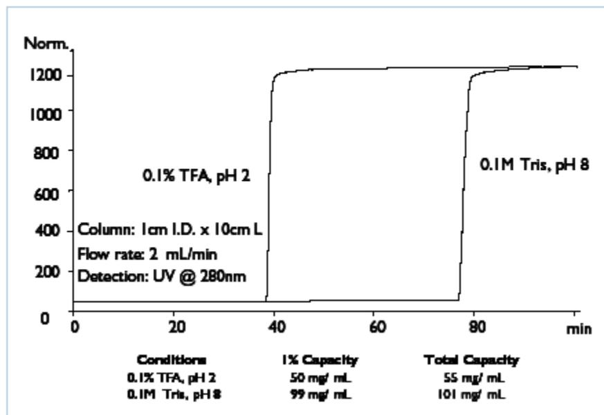
Under basic conditions vancomycin behaves as a more hydrophobic molecule, and the dynamic capacity on Amberchrom XT20 doubles. This demonstrates the advantage of a wider pH range with polymeric resins.
