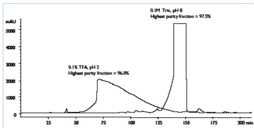
A chromatographic polishing step was developed for vancomycin, (*Sigma USP grade (MW 1485)*). The HPLC purity of the feedstock was ~89%. Preparative purification was performed on a 1cm I.D. x 25 cm L Amberchrom XT20 column under two different pH conditions. An equivalent ACN linear gradient of 3 to 25% over 10 CV was used for each.
