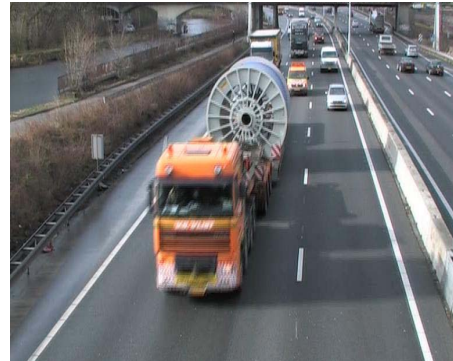
Figure 2: 400kV XLPE drums transported by truck
