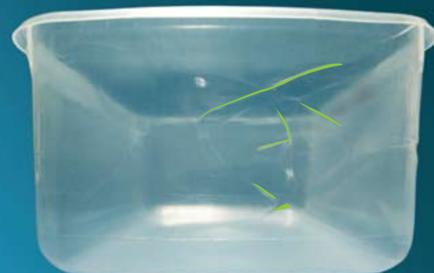
USING C-RCP WITH VERSIFY™ IMPACT MODIFIER No fracture after impact / No stress whitening
