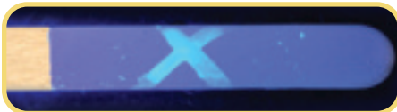
Above: A tongue depressor that has been coated with paint containing Fastrack™ XSR™. The Sodium Hydroxide solution was applied, and is visible under the UV lamp.
