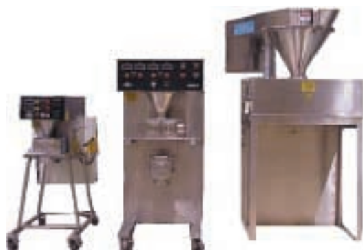
Figure 1. Comparison of laboratory, pilot-plant, and production roll-compaction equipment.
