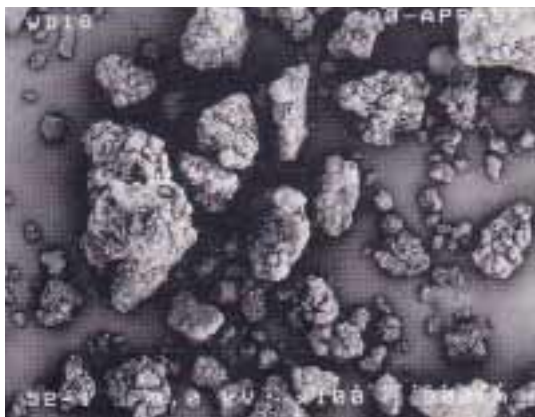
Figure 1. SEM of Polyethylene Oxide (POLYOX WSR)
