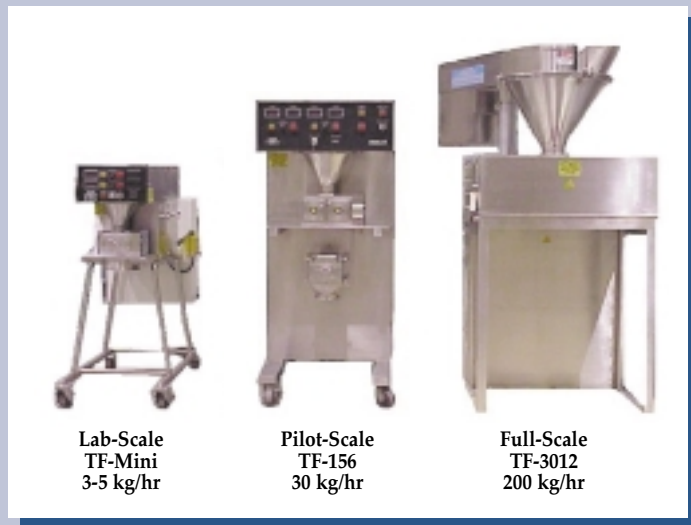
Figure 1: Comparison of Lab-Scale Roll Compaction Equipment (TF-Mini), Pilot-Scale Roll Compaction Equipment (TF-156), and Full-Scale Roll Compaction Equipment (TF-3012)
